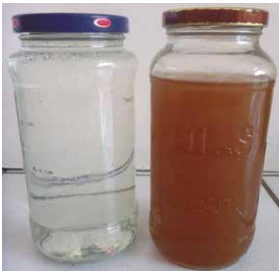
Figure 10. Comparison of 'normal' piped water (left) and 'dirty water' (right) collected by Neff from a tap at his residence in Grand Anse, Grenada. The sample at right qualifies as 'severe'
